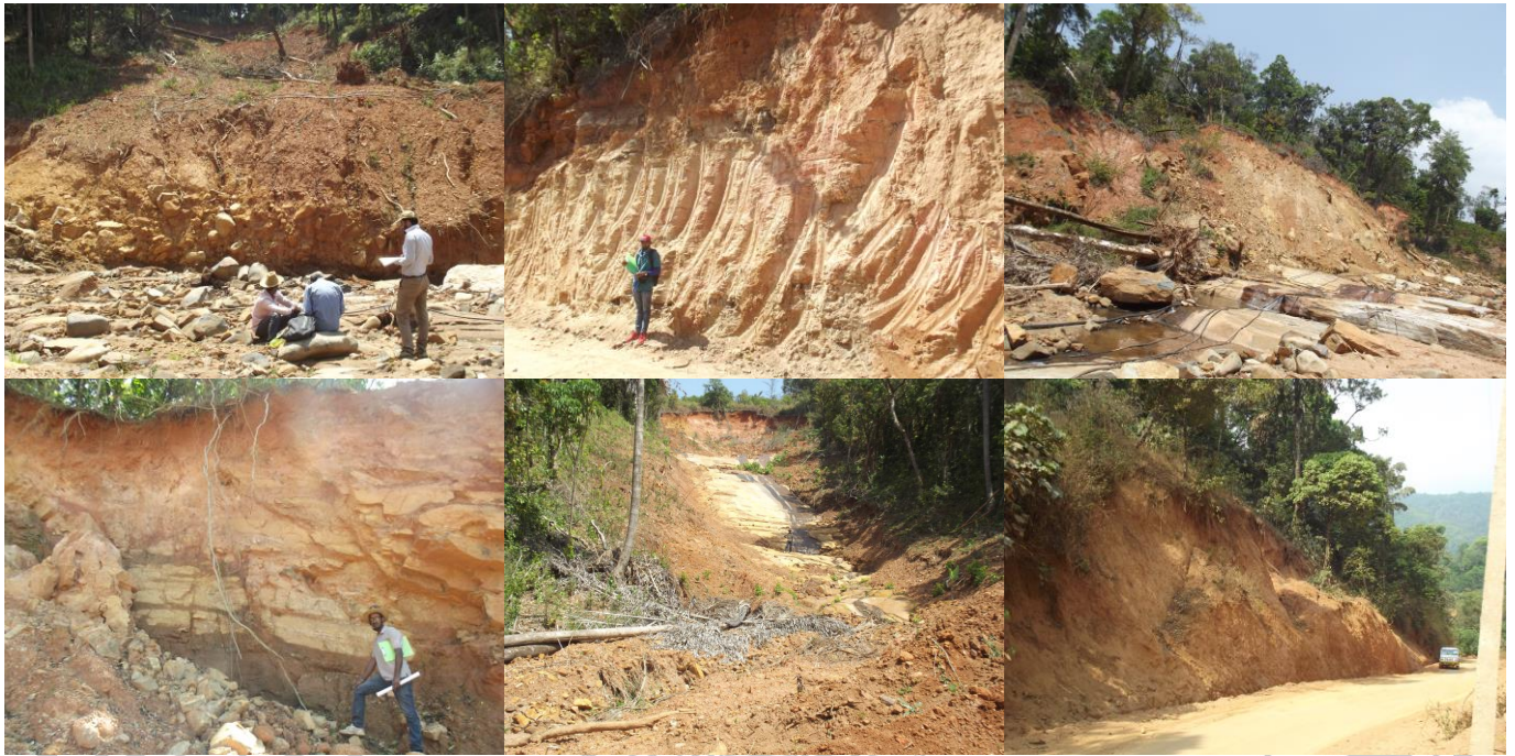
Figure-4.8: Shows field photographs of bedrock surface and overburden thickness sections and cut slopes in different places of study area which became very helpful to assume the overburden thickness
